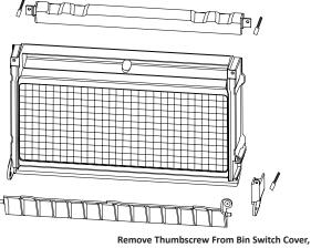
emove Thumbscrew From Bin Switch Cover Support The Damper, and Remove
