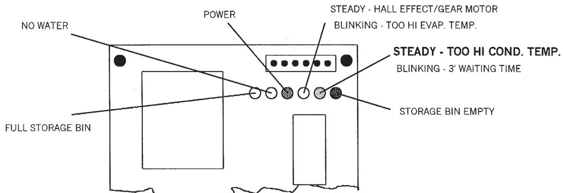
E. Check for the correct CUT-OUT and CUT-IN of the **float reservoir water level sensors** by shutoff the valve on the water supply line. This will cause a gradual decrease of the water level in the float reservoir and as soon as the level gets below the sensors, the flaker stops to operate and the **5th YELLOW warning LED** will glow to signal the shortage of water (Fig.5).
