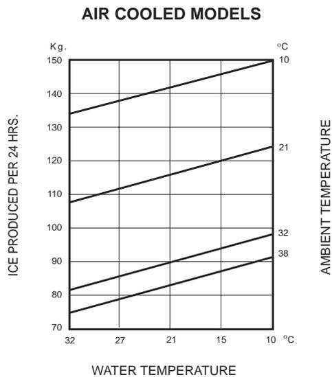
**NOTE.** The daily ice-making capacity is directly related to the condenser air inlet temperature, water temperature and age of the machine.
