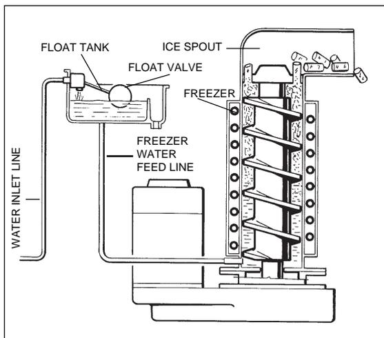
The ice, being constantly lifted up, meets the tooth of the ice breaker which is fitted on the top end of the auger, where it gets compacted, cracked and forced to change from vertical into horizontal motion to be discharged out, through the ice spout, into the storage bin.
