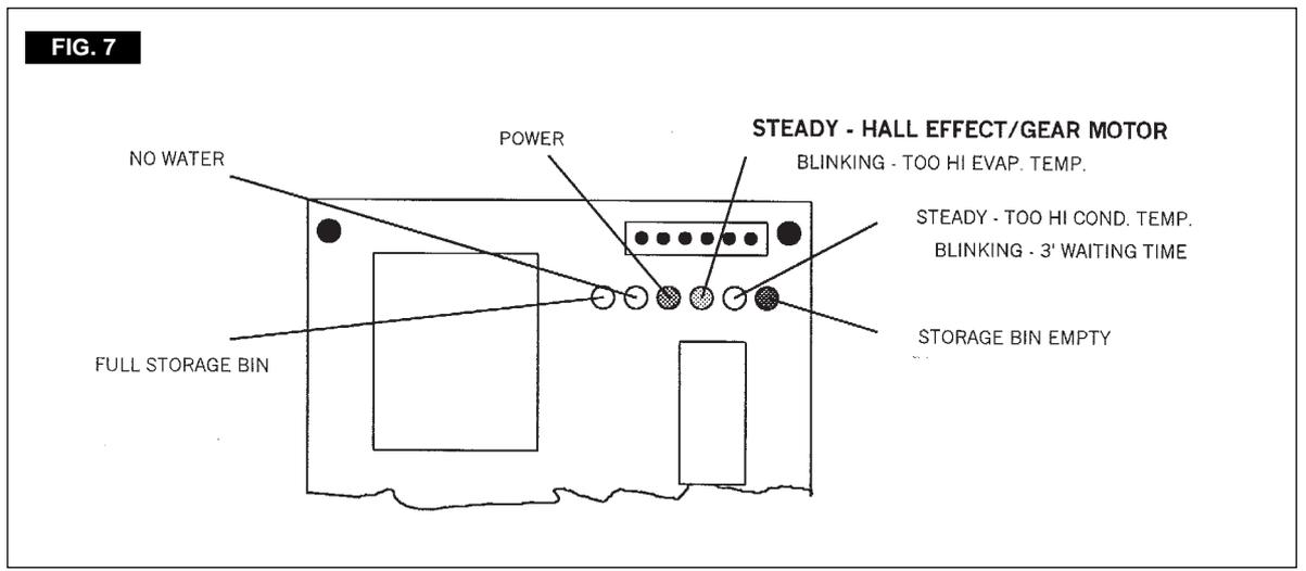
When the gear motor rotating speed is slowed **below 1300 r.p.m.** from the normal speed of 1400 r.p.m. the Electromagnetic Safety Device transmits an electrical signal to the MICROPROCESSOR to **stop immediately** the unit operations like it occurs for the wrong rotation, with the lighting-up of the **3RD YELLOW WARNING LED**. This to relieve from the excessive load all the electrical and mechanical components of the entire Drive System and extend their durability.
